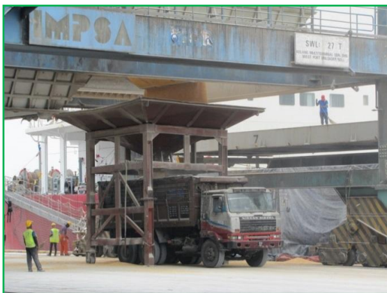
Corn loaded into a hopper into a 30 ton truck (left). Cargill warehouses at Westports facility, Port Klang where grain could also have been transported by conveyor directly from the boat (right).
